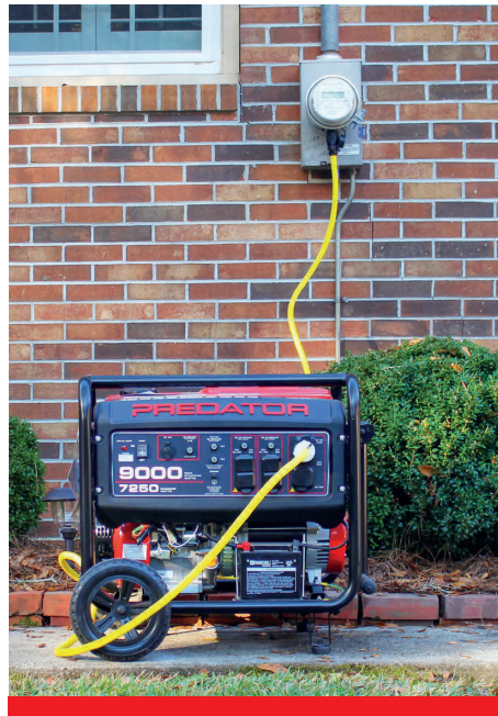
A portable generator is powered by fuel and should not be attached to a circuit breaker, fuse or outlet.
