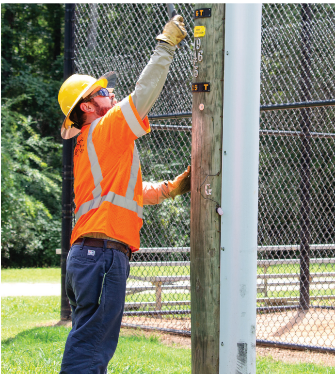
Advanced Line Technician Jacob Riddei checks the condition of a power pole by performing the hammer test. Riddei has to listen for a distinct sound to ensure the pole is not rotting or decaying.
